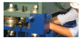
machinery. RotaChock is a mounting chock and we recommend that it not be used as a lifting device.
