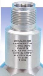
The HS-100I and HS-100SI Series of industrial accelerometers are AC versions which are ATEX and IEC Ex certified for use in Group I and Group II potentially explosive environments. They typically operate over a temperature range of -55 to 140°C and cover a frequency response over 2 Hz to 10 kHz.
