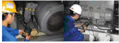
With C911, the automatic condition monitoring, signal analysis and expandable laser alignment capability has never been handy and convenient to maintenance personnel.
